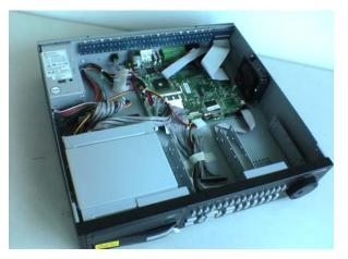
Figure 2: Internal construction of DVR-4TN/8TN/16TN/16TS/16TT
